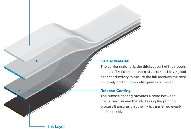
The ink layer is the part of the ribbon that is transferred onto the media. It can be made of wax, resin or a combination of both. It can also contain additives to achieve a better print and colour when needed.
